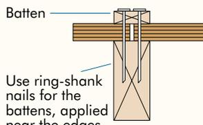
Use ring-shank nails for the battens, applied near the edges in two staggered rows
