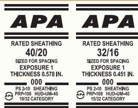
Specially designed for subflooring and wall and roof sheathing. Also good for a broad range of other construction and industrial applications. Can be manufactured as OSB, plywood, or other wood-based panel. BOND CLASSIFICATIONS: Exterior, Exposure 1. COMMON PERFORMANCE CATEGORIES: 3/8, 7/16, 15/32, 1/2, 19/32, 5/8, 23/32, 3/4.
