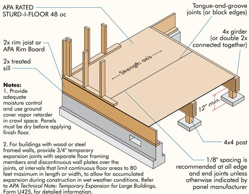
In some applications, particularly in hallways and other heavy traffic areas, greater stiffness in the floor may be desirable. Modifications to the 48-inch framing system, such as addition of straight or diagonal blocking, will increase stiffness considerably.
