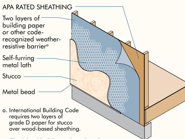
a. International Building Code requires two layers of grade D paper for stucco over wood-based sheathing.
