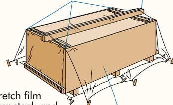
Stretch film over stack and secure to tie-down stakes
