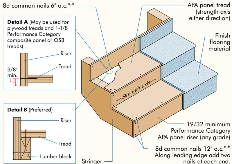
a. Predrill tread end grain at mid-thickness with 3/32" bit. Maintain at least 3/8" edge distance in riser.
