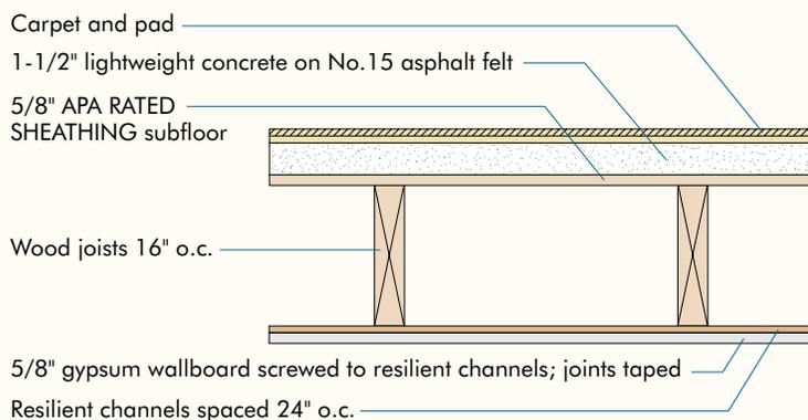
The IIC ratings define the capacity to control impact noise. In most cases, required IIC rating values are about the same as for STC.
