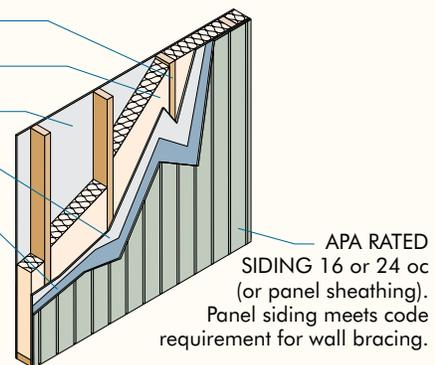
APA RATED SIDING 16 or 24 oc (or panel sheathing). Panel siding meets code requirement for wall bracing.
