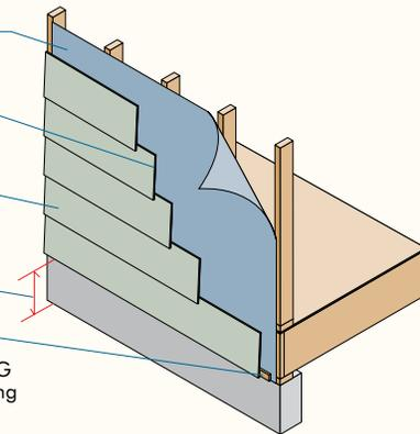
a. For engineered shear wall segments or wall bracing requirements, use APA RATED SHEATHING for wall sheathing under lap siding (see Figure 18). Other methods permitted by model building codes for braced wall segments may also be used.
