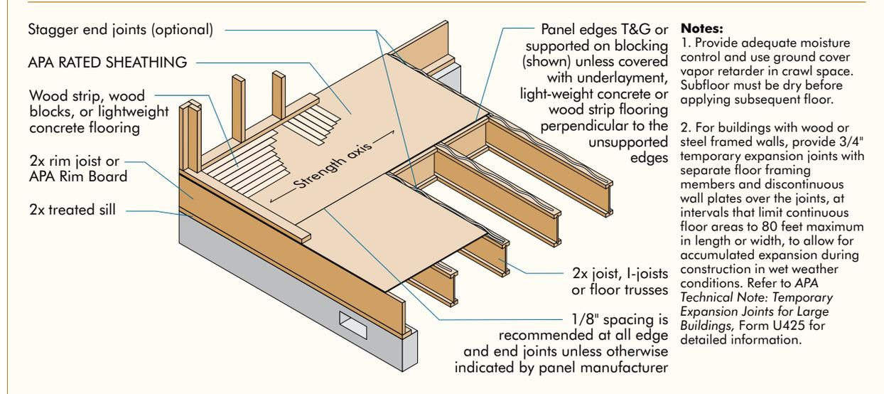
APA RATED SHEATHING Exposure 1 may be used where temporary exposure to moisture or weather is expected during construction. However, only Exterior panels should be used where long-term exposure to moisture or weather will be required. See “Plywood for Outdoor Decks” on page 89 for additional information on permanently exposed panels.
