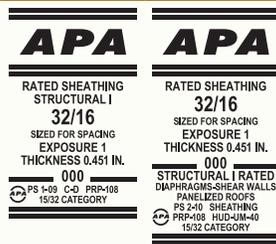
Unsanded grade for use where shear and cross-panel strength properties are of maximum importance, such as panelized roofs and diaphragms. Can be manufactured as OSB, plywood, or other wood-based panel. BOND CLASSIFICATIONS: Exterior, Exposure 1. COMMON PERFORMANCE CATEGORIES: 3/8, 7/16, 15/32, 1/2, 19/32, 5/8, 23/32, 3/4.
