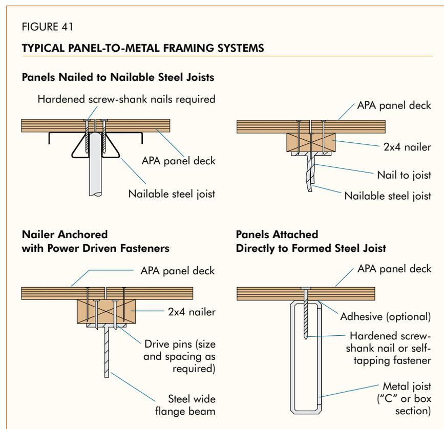
Typical panel-to-metal framing systems are illustrated in Figure 41. Load-span recommendations are the same as for wood-frame systems. For more information, refer to *APA Design/Construction Guide: Wood Structural Panels Over Metal Framing*, Form T625.
