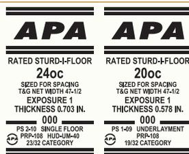
Specially designed as combination subfloor-underlayment. Provides smooth surface for application of carpet and pad and possesses high concentrated and impact load resistance. Can be manufactured as OSB, plywood, or other wood-based panel. Available square edge or tongue-and-groove. BOND CLASSIFICATIONS: Exterior, Exposure 1. COMMON PERFORMANCE CATEGORIES: 19/32, 5/8, 23/32, 3/4, 7/8, 1-1/8.
