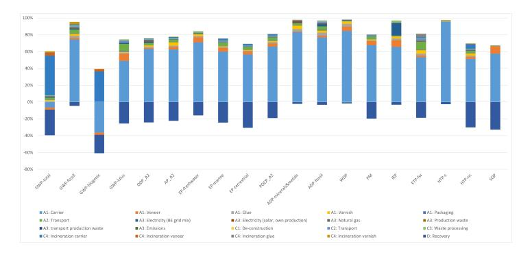
To visualize which materials and processes give the largest contribution to the environmental indicators a major contributions analysis has been included. In the graph below the total value of each indicator has been set to 100 %. The colours indicate which part of the environmental effects are caused by the different materials and processes in the life cycle of the veneered products.
