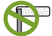
For hanging signs, use a clevis and pin attachment. Do not use mounting bolts into the edge.
